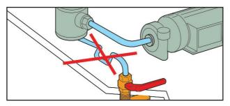
strainer and pump intake should be connected without siphoning; the piping should always rise from the water intake until the pump intake.
