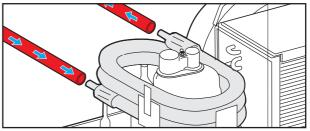
or plastic hose. The flow sense is marked with arrows; anyhow the water enters from the bottom coil of the heat exchanger and goes out from the top outlet. Hose routing should avoid siphoning which will prevent the pump to prime. The over board outlet port should be as low as possible but above the water line: this to limit the water discharge noise and to avoid horizontal jets.
