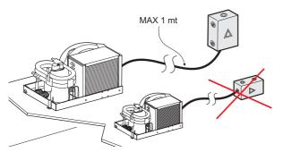
The connection box must be installed vertically on a bulkhead near the conditioner unit to which is linked with 1 m long cables. Cables should enter from bottom side and should be fastened by means of plastic strippers.
