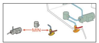
The intake line should be as short as possible (it is very difficult to run a good circuit with an intake piping longer than 1 m).
