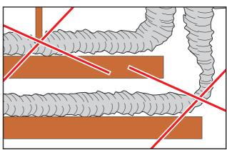
The unit efficiency is strictly related to the air flow. Thus it is important to have an air distribution without weak points, keeping the original suggested diameter, and not exceeding the suggested duct length.
