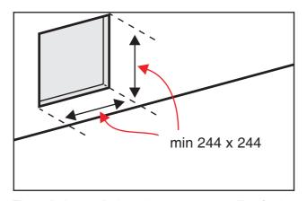
The unit draws air through one or more grills of adequate dimensions. Minimum dimensions of return grill are 244x244 regardless to unit capacity. The return air should be straight to the unit: if return air ducting is needed, please contact our technical service.
