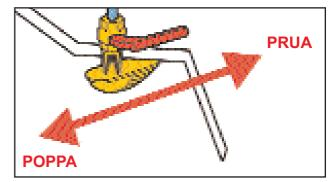
The water intake must be "scoop" type oriented forward.
