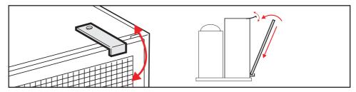
The unit draws air through the refrigerant-ambient air heat exchanger which has arrow aluminium fins. These fins so close would get soon clogged because of dust and dirty if not installed directly on the exchanger as shown in the drawing below. The air filter needs periodical maintenance and must be accessible for service.
