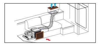
A.- The unit is engineered to draw directly the ambient air, then the unit should be installed in one of the cabins to be conditioned (only the evaporator assy in case of Split models).
