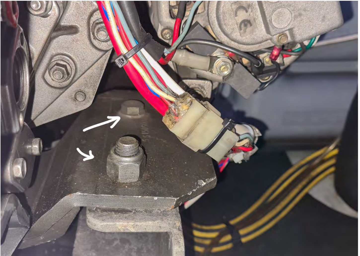
Aft port bolts that hold the engine to the steel frame
