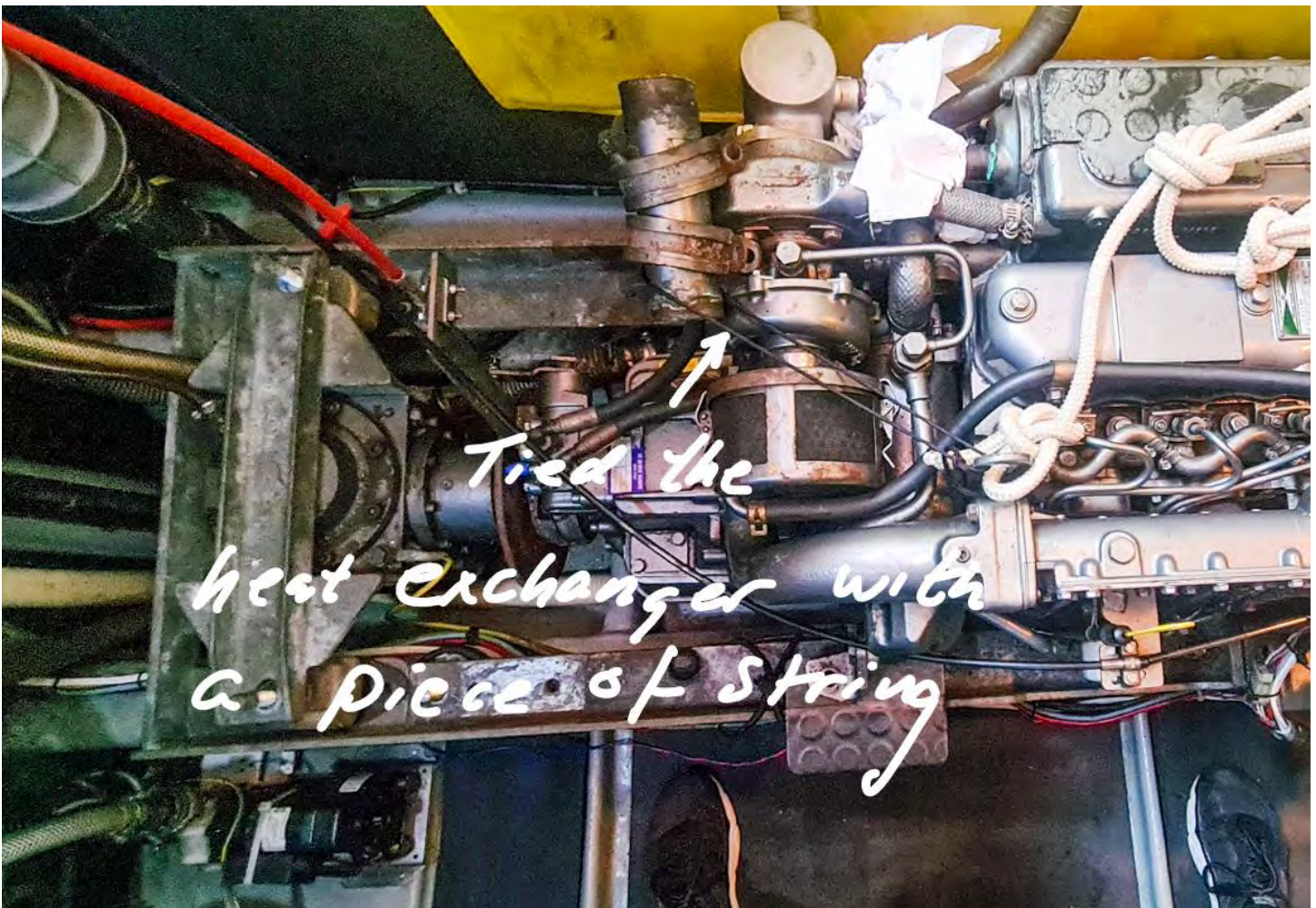
Tied the heat exchanger to the top of the engine to get it out of the way without disconnecting the hoses
