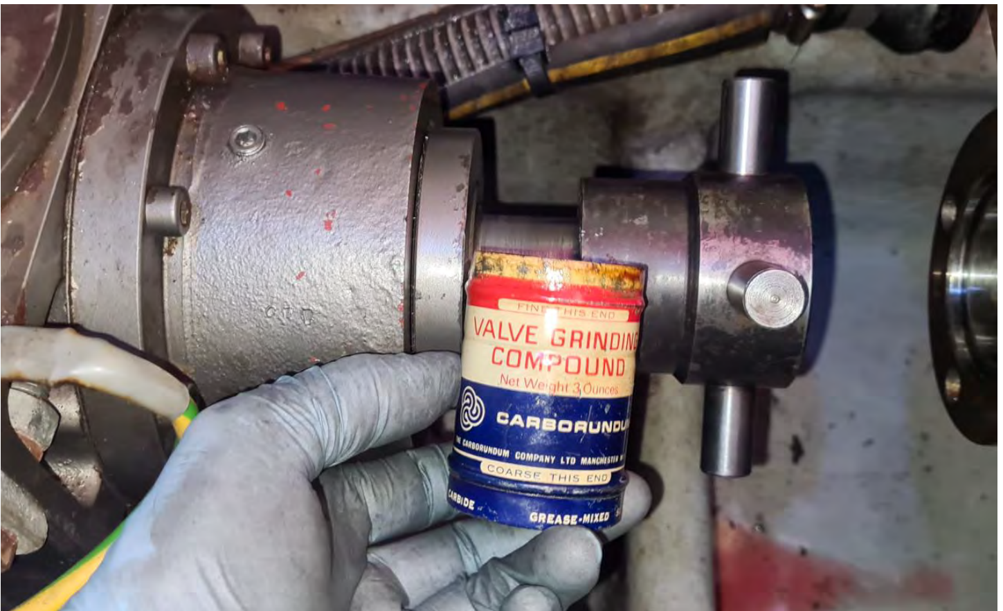
Final step of the honing done with valve grinding paste directly on the shaft. Super smooth fit.
