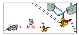
The intake line should be as short as possible (it is very difficult to run a good circuit with an intake piping longer than 1 m).
