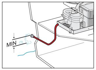
C.- Treating the ambient air means the separation of condensate produced by air humidity. His condensate must be drained and discharged over board; this means that the unit should be installed at a certain level to be connected to an outlet port, considering that the condensate hose must have a minimum heeling.
