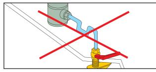
strainer and pump intake should be connected without siphoning; the piping should always rise from the water intake until the pump intake.
