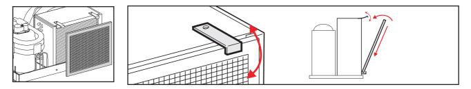
The unit draws air through the refrigerant-ambient air heat exchanger which has arrow aluminium fins. These fins so close would get soon clogged because of dust and dirty if not installed directly on the exchanger as shown in the drawing below. The air filter needs periodical maintenance and must be accessible for service.
