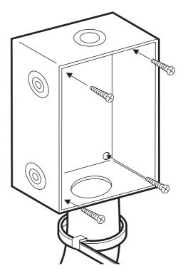
The connection box has four holes in the base to be used for fastening screws.
