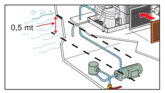
The pump should be installed with the sheft in horizontal position and the water outlet on the top or at least 50 cm below the floating level.
