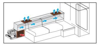
B.- The treated air (blown by the fan) should be connected to one or more delivery grills by means of flexible ducts or using a yacht structure as a duct. Duct must be properly insulated.
