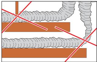
The unit efficiency is strictly related to the air flow. Thus it is important to have an air distribution without weak points, keeping the original suggested diameter, and not exceeding the suggested duct length.
