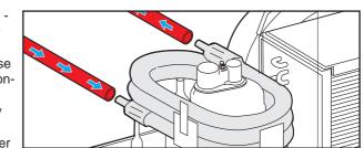
or plastic hose. The flow sense is marked with arrows; anyhow the water enters from the bottom coil of the heat exchanger and goes out from the top outlet. Hose routing should avoid siphoning which will prevent the pump to prime. The over board outlet port should be as low as possible but above the water line: this to limit the water discharge noise and to avoid horizontal jets.
