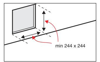
The unit draws air through one or more grills of adequate dimensions. Minimum dimensions of return grill are 244x244 regardless to unit capacity. The return air should be straight to the unit: if return air ducting is needed, please contact our technical service. 2.9.B - Air delivery
