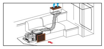
A.- The unit is engineered to draw directly the ambient air, then the unit should be installed in one of the cabins to be conditioned (only the evaporator assy in case of Split models).
